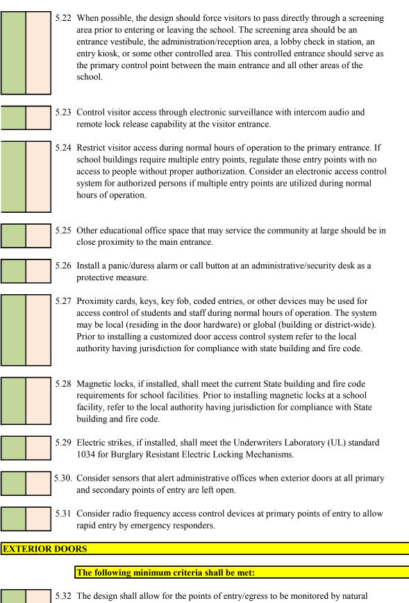
2 The design shall allow for the points of entry/egress to be monitored by natural and/or electronic surveillance during normal hours of operation and during special events.
